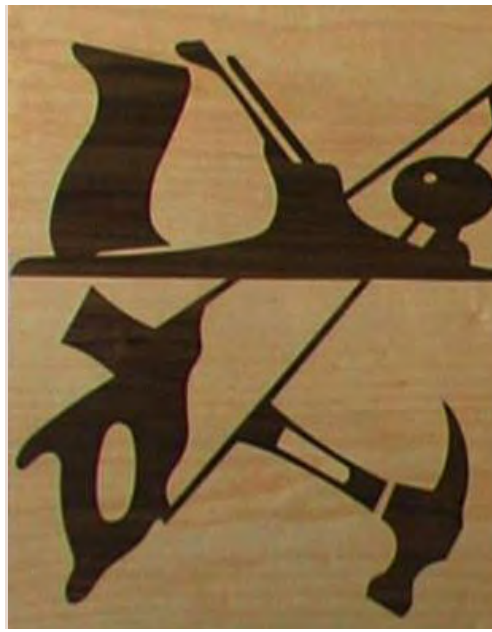
Custom-made sign using inlaid laser cutting technology. Customer's own design used.
